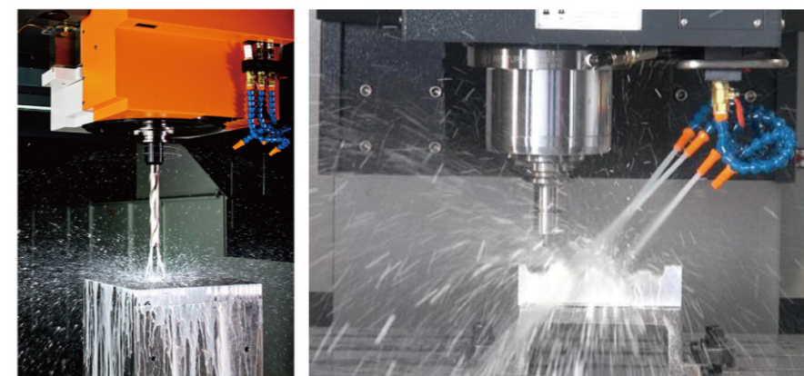
● Coolant through spindle (Opt.) ● Cutting fluid system (Std.)
